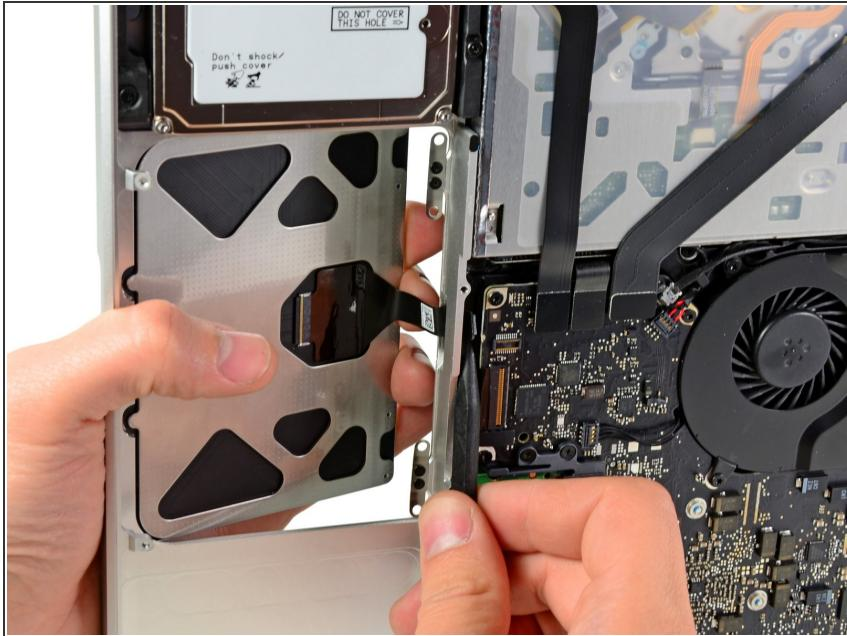
ⓘ If you are installing a replacement trackpad that didn't come with the attached flex cable, you'll need to use the cable from your old trackpad.
